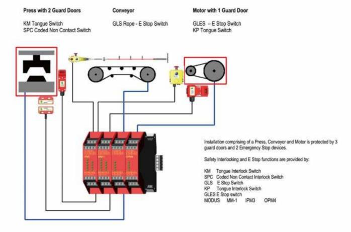
B. Monitoring of 2 guard doors and 3 emergency stop buttons, interruption of 3 drives, grouping in 2 groups with higher-level stop switch
