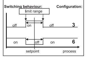
on: Relay "activated" off: Relay "not active"
