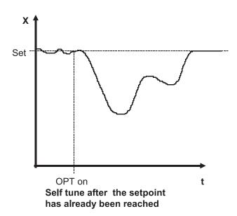
Self-tuning can be stopped by selecting the option OPT = OFF and pressing the "E"-key.
