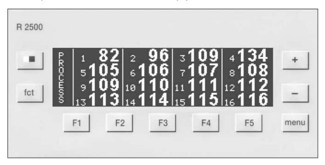
The device is operated by menus. The different parameters are displayed mainly in clear and can be displayed in various languages.
