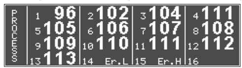
Zone 13: Actual process value 113 °C Zone 14: Sensor error: lower than Zone 15: Sensor error: Zone 16: Zone switched off
