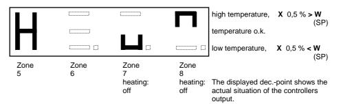
Zone 5: H = Manual output ratio. Flashing: sensor error (see page 14)
