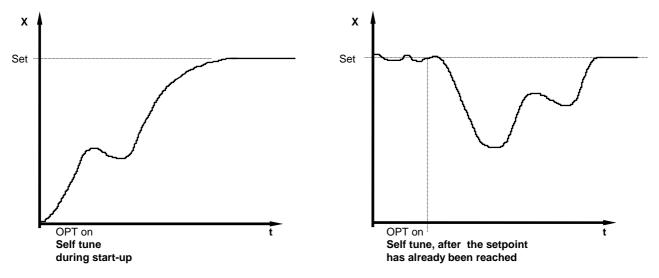
Self-tuning can be stopped by selecting the option  $\ \ \, \mbox{OPT} = \mbox{OFF}$  and pressing the "E" - key.
