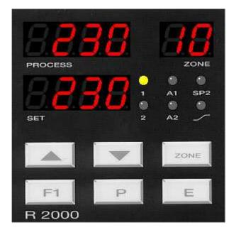
**LED 1:** Control output "heating" of the choosen zone active **LED 2:** Out of operation
