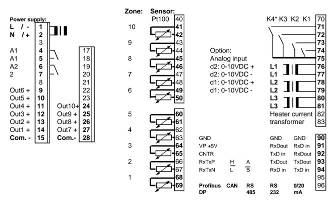
It is not permitted to connect the grounds of the sensor-inputs and bist. voltage-outputs with each other.
